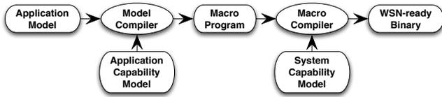
Fig. 1. Compiling business process models into WSN-executable code.
